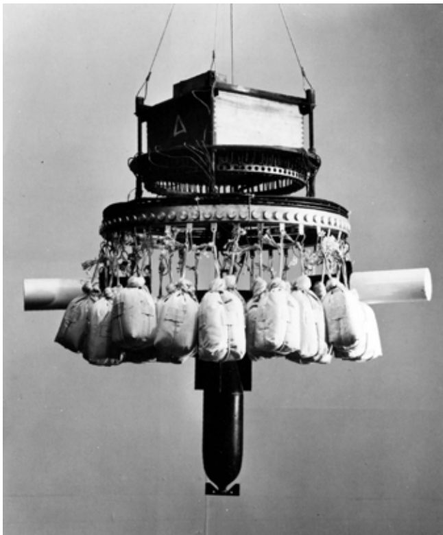
Each balloon carried sandbag ballasts, two incendiary bombs and an anti-personnel bomb.
